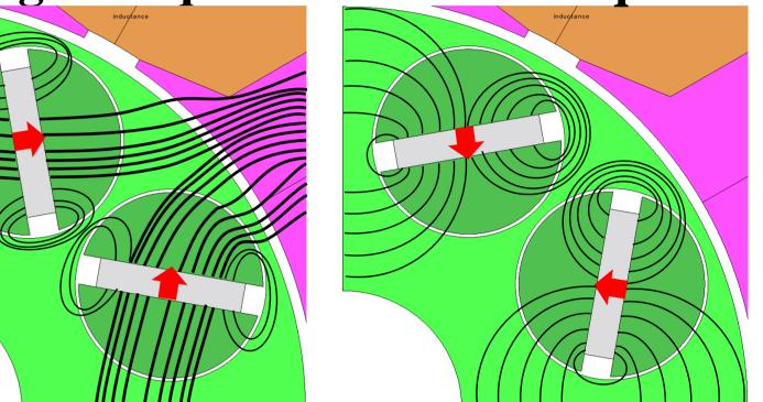
> Short-circuit magnetic flux in the rotor varies with the magnet angle > Changes in magnet angle cause variations in armature cross flux,
